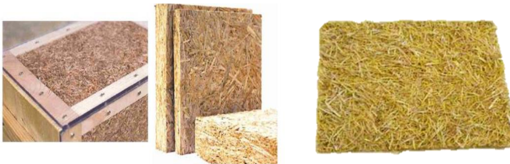
Figure 9. Left: Blow-in insulation material from 100% cattail in a display case, and construction panels made of cattail. Source: (Colbers et al., 2017). Right: Fibermat typha (Wuzella et al., 2011)
